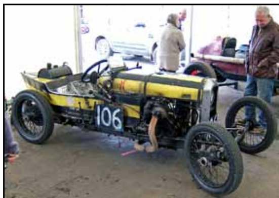
The GN (HR Godfrey & Archibald Frasier-Nash) 'Thunderbug'. Note 4.3 liter V twin engine!
