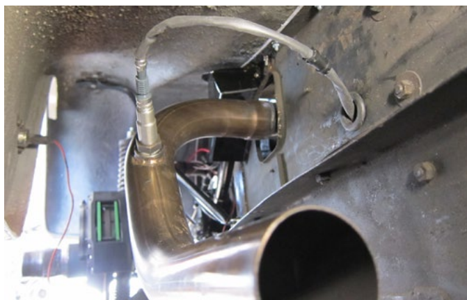
The harness in the left inner wing connecting the sensor on the manifold to the ECU
