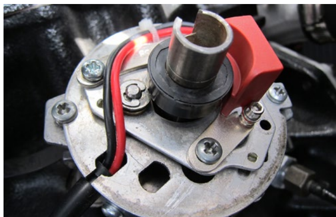
The Hall Effect sensor installed in the distributor
